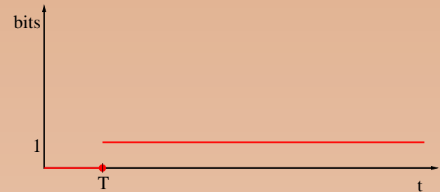
Step function: u_T(t) = \begin{cases} 0 & \text{for } t \leq T \\ 1 & \text{for } t > T \end{cases}
