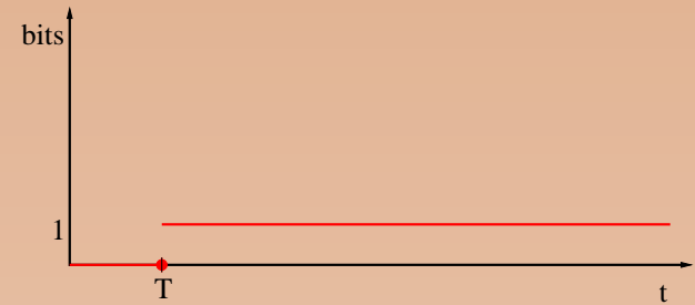
Step function: u_T(t) = \begin{cases} 0 & \text{for } t \leq T \\ 1 & \text{for } t > T \end{cases}
