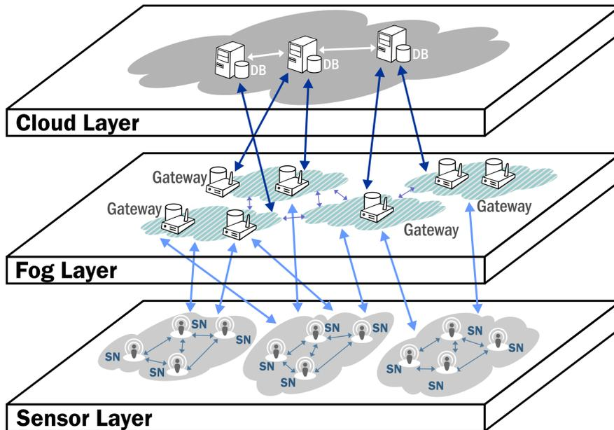
Fig. 2 High level overview of fog based IoT
