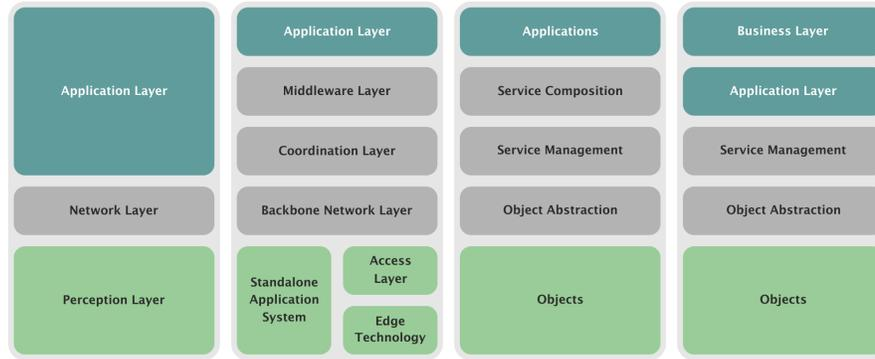
**Fig. 1** IoT architecture proposals (3-layers and 5-layers) [5]
