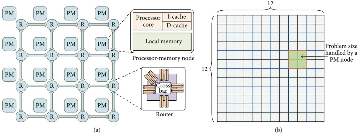
FIGURE 1: (a) Sketch map of homogenous OLPCs and (b) an example of data partitioning of data-parallel applications.
