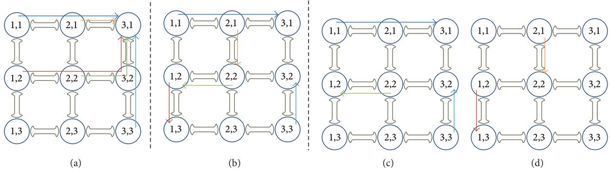
FIGURE 5: Examples of communications in a  $3 \times 3$  2D-mesh network.
