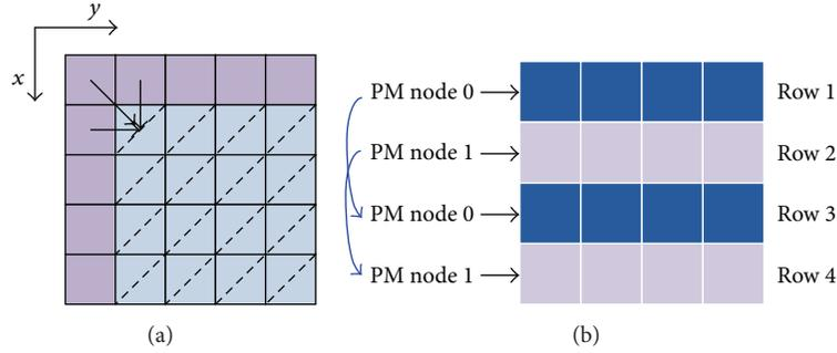
FIGURE 9: (a) Wavefront Computation; (b) its parallelization.
