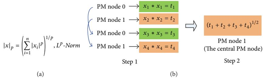
FIGURE 10: (a) Vector Norm and (b) its parallelization.
