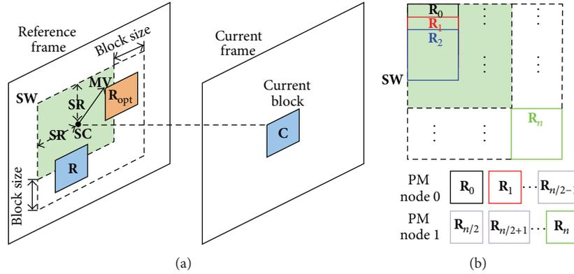
FIGURE 11: (a) Block Matching Algorithm in Motion Estimation and (b) its parallelization.
