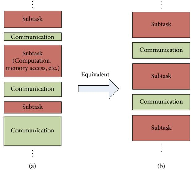
FIGURE 2: The subprogram running on a processor node is abstracted as a set of subtasks and communications.
