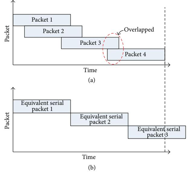
FIGURE 3: Packets in a communication issued by a processor node.
