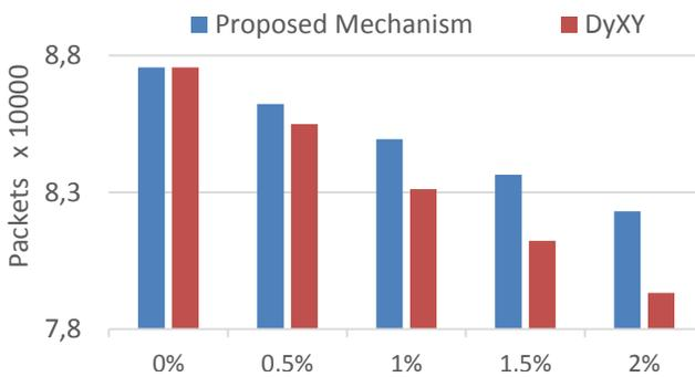
Fig. 10 Fault-tolerant capability under Bit-Reversal Traffic
