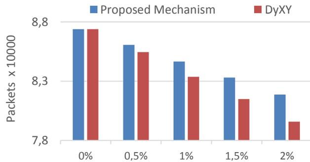
Fig. 8 Fault-tolerant capability under Transpose1 Traffic
