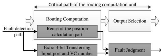
Fig. 2 Block diagram of the fault detection
