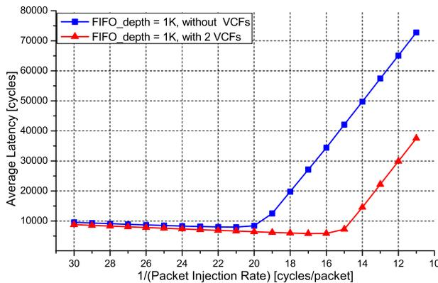
Figure 7. Latency measurement results (reconfiguration time = 10  $\mu$ s)
