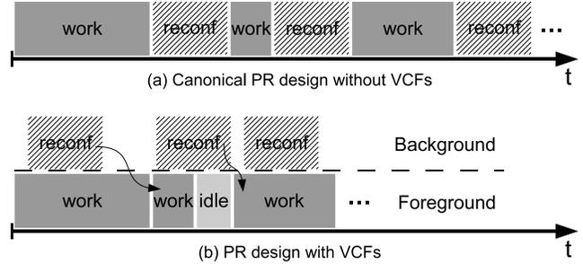
Figure 2. Timing diagrams of PR designs without or with VCFs
