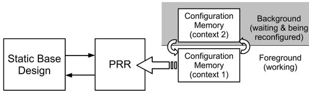
Figure 1. Virtual reconfigurations on multi-context FPGAs
