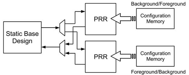
Figure 3. Virtual reconfigurations on single-context FPGAs
