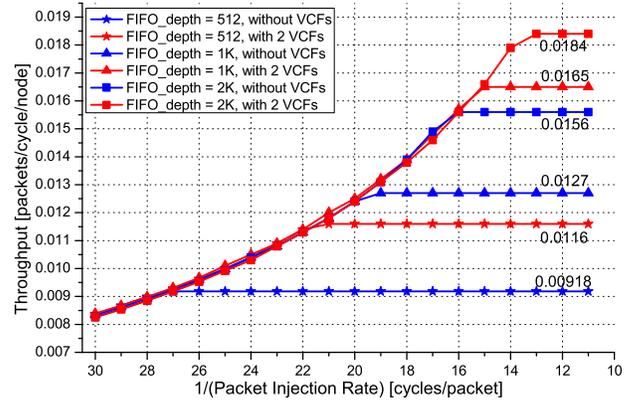
Figure 5. Throughput measurement results (reconfiguration time = 10  $\mu\text{s}$ )
