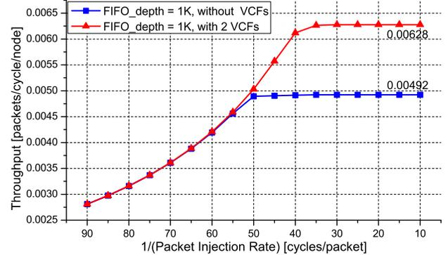
Figure 6. Throughput measurement results (reconfiguration time = 50  $\mu\text{s}$ )
