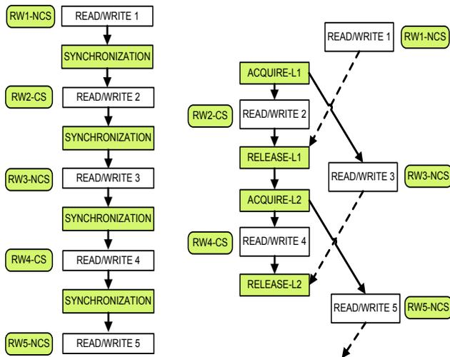
**Figure 7. a) Weak Ordering      b) Release Consistency**
