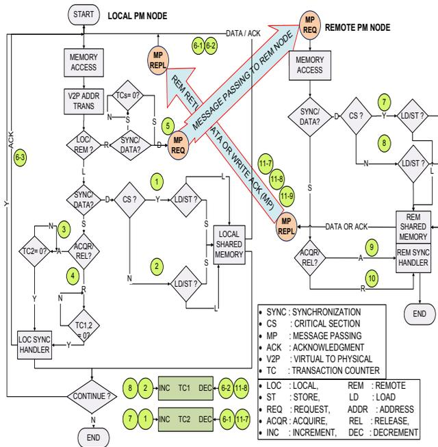
Figure 8. Transaction counter based release consistency
