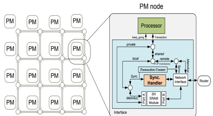
Figure 3. NoC platform for weak memory consistency
