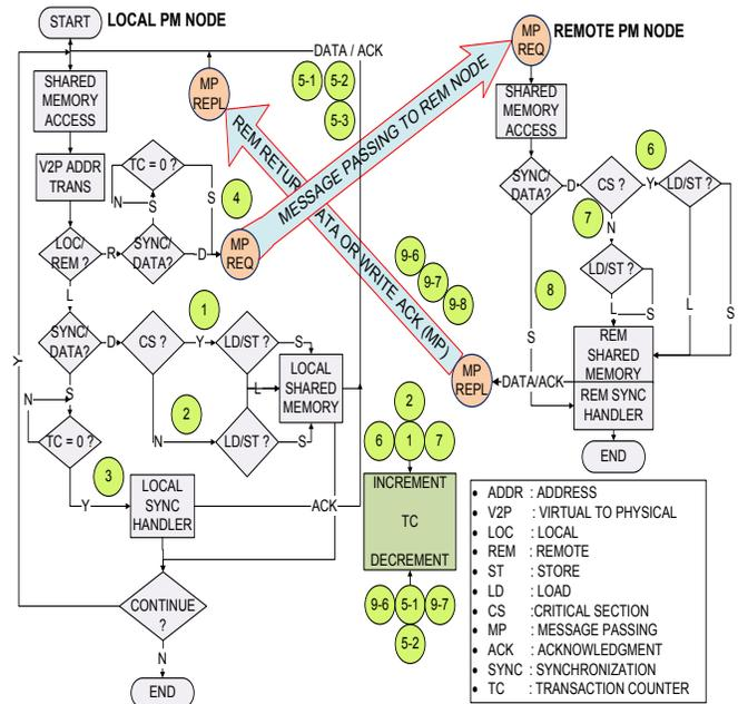
Figure 5. Transaction counter based weak consistency
