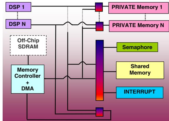
Fig. 9. Crossbar architecture with STBus interconnect. Low-bandwidth slaves have been grouped to the same crossbar branch (partial crossbar concept).
