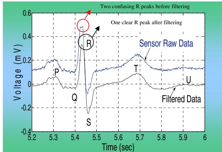
**Fig. 5.** ECG raw and filtered data (lead I)
