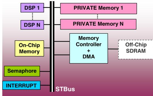
Fig. 8. Single bus architecture with STBus interconnect
