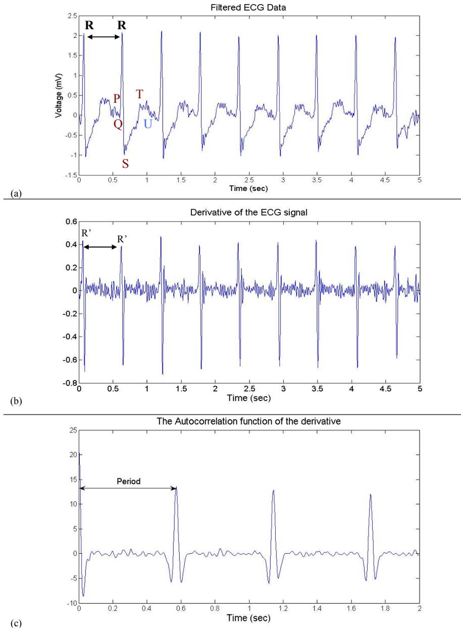
**Fig. 6.** Heart period analysis: (a) ECG signal peaks P, Q, R, S, T, and U; (b) derivative amplifying R peaks; (c) autocorrelation of the derivative characterized by significant periodic peaks having the same value as the period of the ECG signal in (b) and thus (a)
