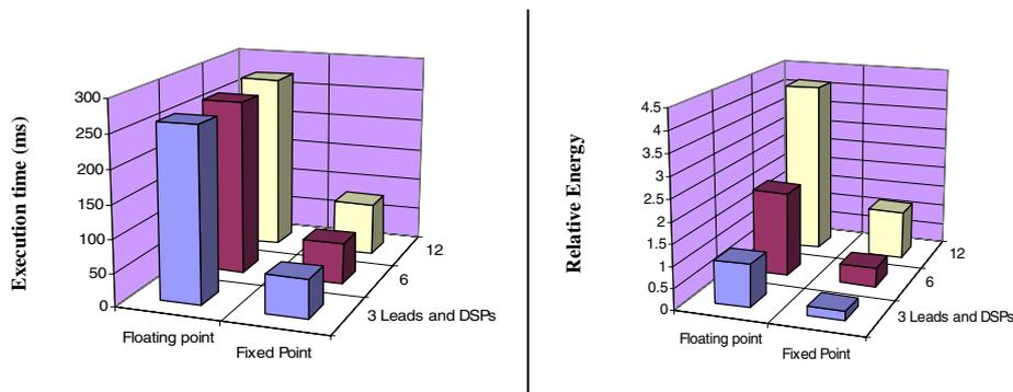
**Fig. 10.** Comparison between different code implementations for the analysis of the 3-lead, 6-lead and 12-lead ECG. Data analysis for each lead is computed on a separate processor core. Sampling frequency of input data was 250Hz. System operating frequency was 200 MHz.
