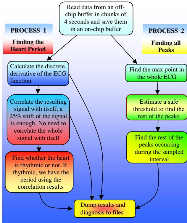
Fig. 7. The Autocorrelation function-based methodology for ECG analysis
