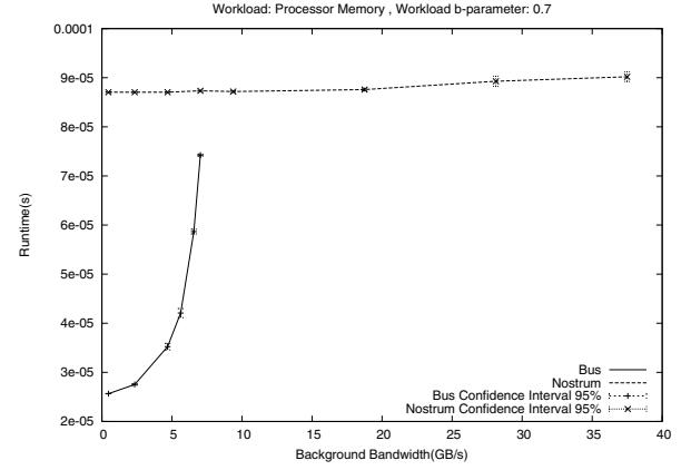
**Figure 8. Runtime as a function of background bandwidth for Nostrum and the bus in the Processor - Memory pattern.**
