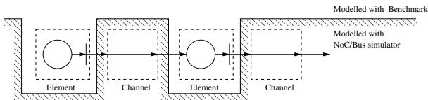
**Figure 2. The channels in the workload model are executed in an interconnect simulator.**
