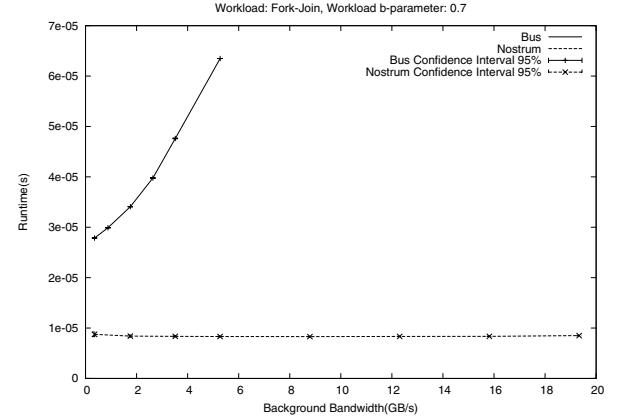
**Figure 10. In the fork-join pattern, the background bandwidth has a similar impact as before but the NoC is always faster than the bus.**
