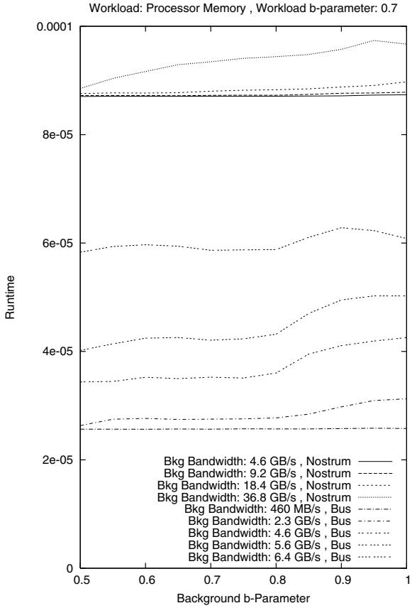
**Figure 7. Impact of the burstiness of background traffic in the Processor - Memory pattern.**
