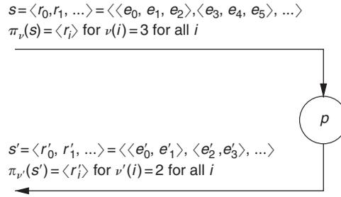
**FIGURE 4.2** The input signal of process  $p$  is partitioned into an infinite sequence of subsignals each of which contains three events, while the output signal is partitioned into subsignals of lengths 2.
