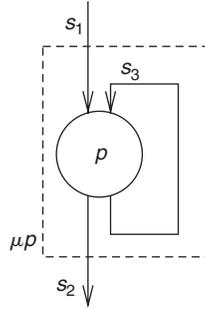
FIGURE 4.3 Feedback composition of a process.
