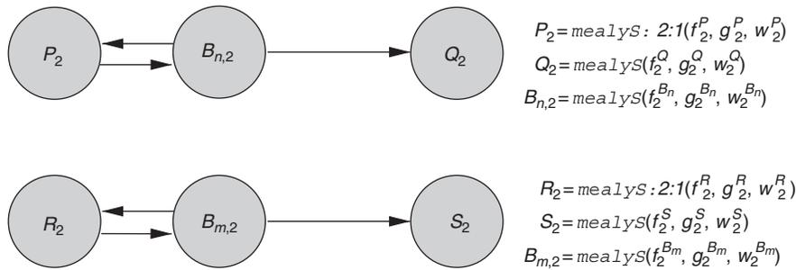
FIGURE 4.9 Two independent process pairs with explicit buffers.
