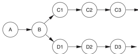
FIGURE 4.1 Over synchronization between functionally independent subsystems.
