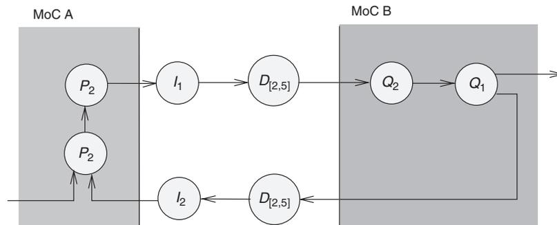
FIGURE 4.7 The channel delay can vary between 2 and 5 cycles measured in MoC B cycles. (From A. Jantsch. Modeling Embedded Systems and SoCs. Morgan Kaufmann Publishers, 2004. With permission.)
