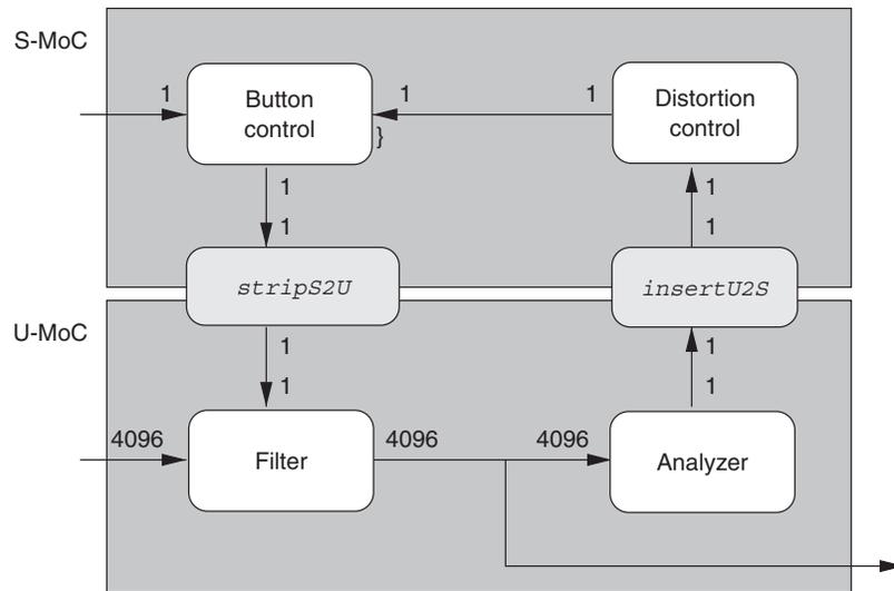
**FIGURE 4.4** A digital equalizer consisting of a dataflow part and control. The numbers annotating process inputs and outputs denote the number of tokens consumed and produced in each evaluation cycle. (From A. Jantsch. Modeling Embedded Systems and SoCs. Morgan Kaufmann Publishers, 2004. With permission.)
