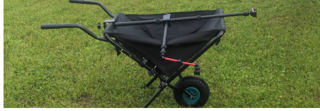
Figure 3: Wheelbarrow and telescopic arm for capturing images in the potato fields.
