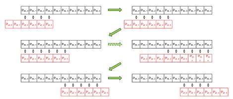
Figure 6: An actual flight path is shifted over a database trajectory to find the place where the sum of all Euclidian distances is the smallest. A predefined parameter decides how many of the actual flight positions (paf) are allowed to be outside of the database trajectory.
