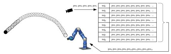
Figure 1: The Transport-by-Throwing approach deals with a robot arm that catches thrown objects with the help of a prediction based on stored trajectories.
