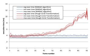
Figure 9: Execution times of the Hough Circle Transformation and the RANSAC algorithm for each frame of an entire flight.
