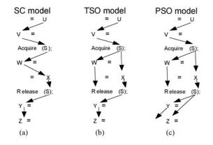
Fig. 1. Comparison of SC, TSO, and PSO models.
