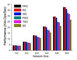
Fig. 13. Performance under bit count application.
