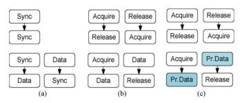
Fig. 4. Global orders: (a) WC; (b) RC; (c) PRC, Pr. data: protected data.
