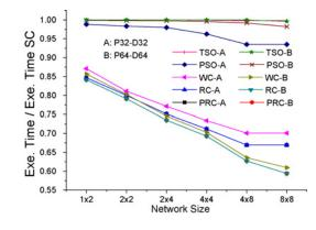
Fig. 14. Pattern search: Ratio (execution time of relaxed models/SC model).
