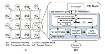
Fig. 8. (a) Homogeneous McNoC. (b) PM node.
