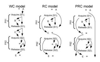
Fig. 5. Non-overlapped protected section, protected data: B, D, and unprotected data: A, C, E.
