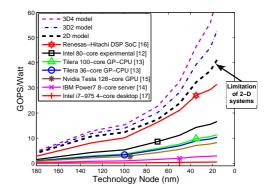
Figure 3: The Effective Computational Efficiency of recent multi-core processors [11, 10, 12, 13, 14, 15] (where markers indicate actual performance data) compared to our model.
