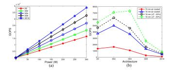
Figure 5: (a) The maximum throughput for our topologies constrained by power and (b) The maximum throughput with a thermal ceiling of 100°C and 100 W. Dashed lines show additional heat removal beyond conventional air cooling
