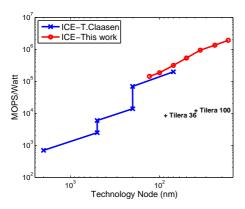
Figure 2: The Intrinsic Computational Efficiency of Silicon, where the the entire die area is filled with 32-bit adders. The difference between T. Claasen's projection and ours lies in the architecture of the 32-bit adder, leading to a minor difference in the energy/operation
