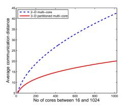
Figure 1: The average geometric distance for a multi-core system for a 2-D and a 3-D realization.
