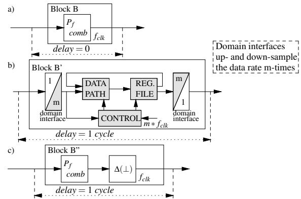
Figure 1: Resource sharing leads to several clock domains and adds an extra delay at the system level.
