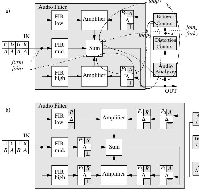
**Figure 6: Audio equalizer: a) initial model b) after the clock domain refinement of the process  $FIR_{low}$**
