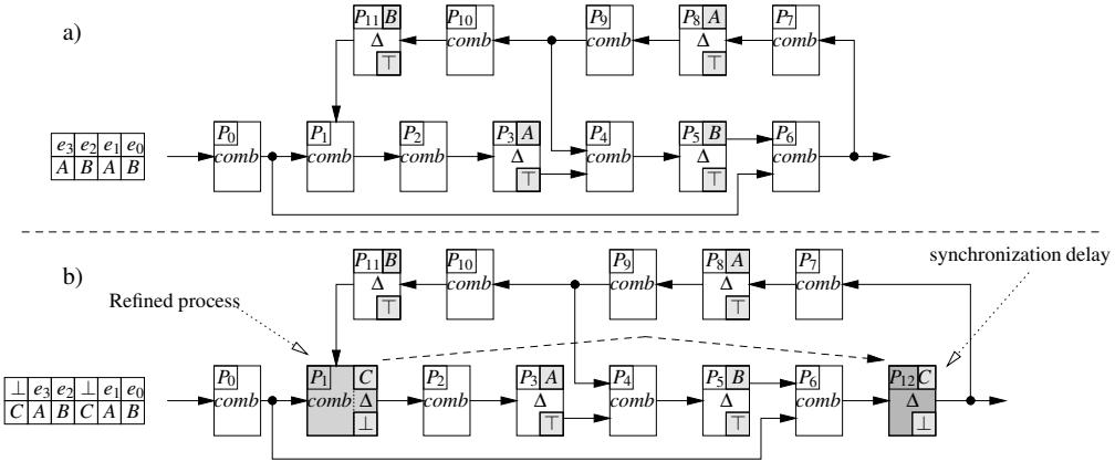
**Figure 4: Synchronization example : (a) initial model after labeling and (b) refined model**
